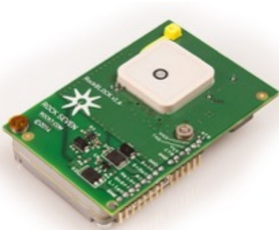
RockBLOCK with built-in patch antenna
